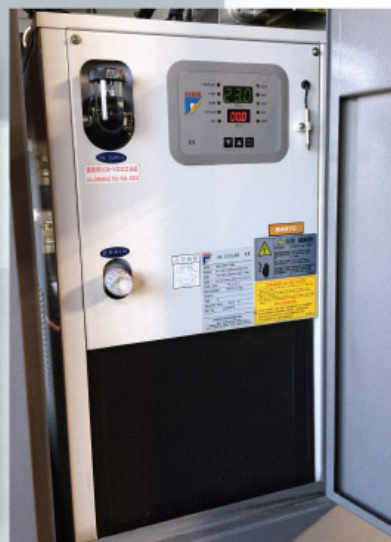
Spindle oil cooler system
