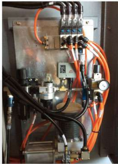
Lubrication and Pressure System
